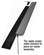
b) Align end of rubber edge with matching channel in bottom section of aluminum blade and slide in until flush at both ends.
