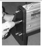
b) Tighten all bolts until rubber begins to compress to blade.
