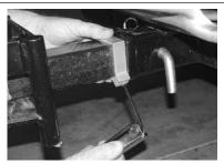
b) Push set collar tight against receiver - hold and tighten set screw with 3/16 allen wrench.
